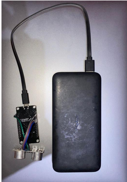
Gambar 4.4 NodeMCU ESP8266 + HC-SR04 + Powerbank
